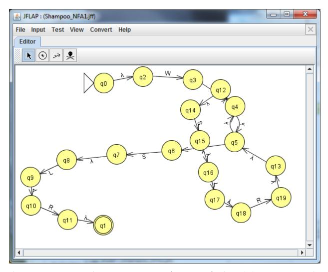
The next step is to convert this NFA to a DFA. Again, if you are not familiar with this process, review the module on converting NFA to DFA. Change the diagram layout to make it more readable. You should have the DFA below.
